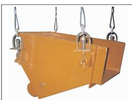
Electromechanical vibrating feeders uses vibratory motor to generate the excitation. There can be combination of one or two vibrator excitor depending on applications.
