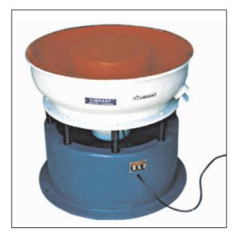
Virtually any machining operation, turning, milling, facing, boring, drilling, shaping, punching, etc. leaves burr or sharp edge on the component. If these components are manufactured in bulk on production basis, they need fast deburring techniques. The solution is
