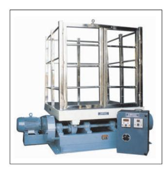
The vibration simulator machine is designed to scientifically simulate the vibrations and jolts subjected to various filled containers during the transportation, within the laboratory. The machine is based on the guidelines provided an ASTM D-999: TAPPI T-S17-pm: and IS702S (part II).
