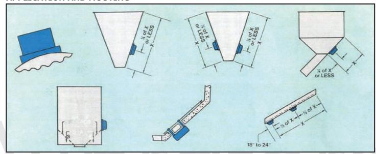
The most ideal installation of vibrator is at 1/4 or 1/3 of its slope length of hopper from the discharge. If more than one vibrators are required to be installed on one hopper they should be equally apart and should be connected in the same phase of supply.
